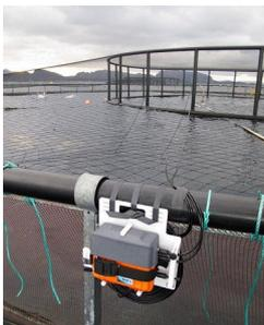
A data collection unit placed at a fish farm. The data is collected via the black cables. (Photo: Nortek)
